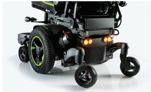
MWD: Drive wheels are directly under the wheelchair with four castor wheels on the ground – two in front of the drive wheel and two behind the drive wheel. A tight turning radius means a MWD chair is ideal for indoor use.
