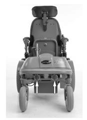
Figure 4. Rear Lights and Reflectors.
