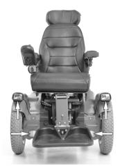
Figure 3. Front Lights and Reflectors.
