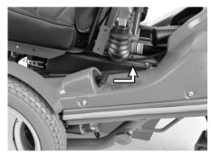
Figure 93. Brake release lever
