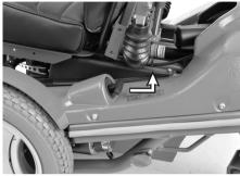
Figure 88. Brake release lever.
