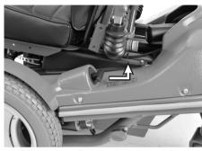
Figure 79. Releasing the brakes
