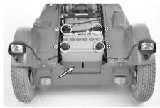
Figure 97. Battery connections and spacer plate.
