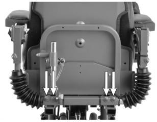
Figure 16. Distance between the arm rests
