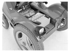
Figure 6. Batteries.
