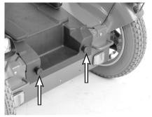
Figure 96. Knobs holding the front cover.
