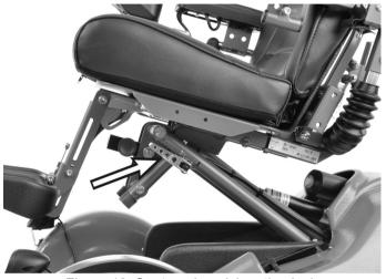
Figure 12. Seat angle quick-acting lock.
