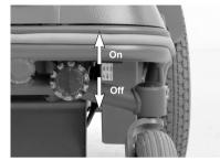
Figure 98. Resetting the main fuse.
