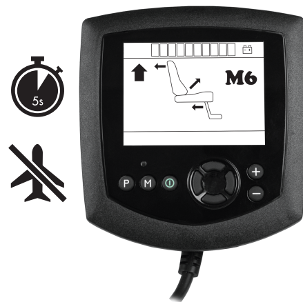
Figure 123. Give and hold a forward command for 5 seconds. Airplane mode is off.
