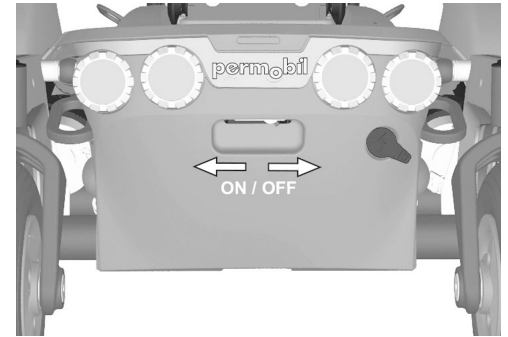
Figure 25. Main circuit breaker.
