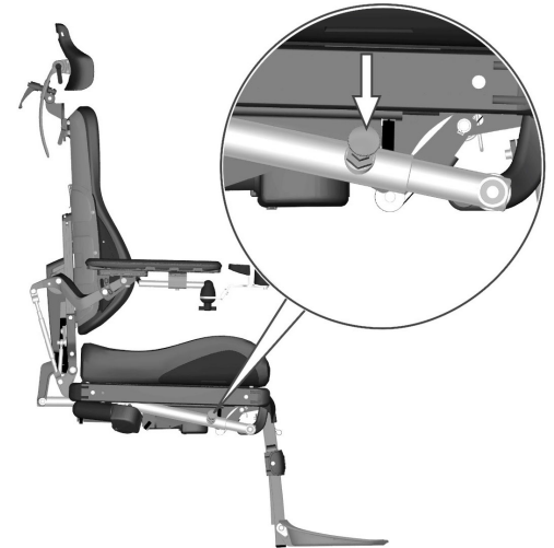
Figure 20. Manually adjusting leg rest angle.
