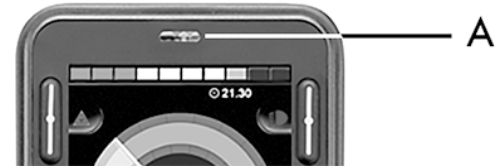
Figure 67. The IR receiver location.
