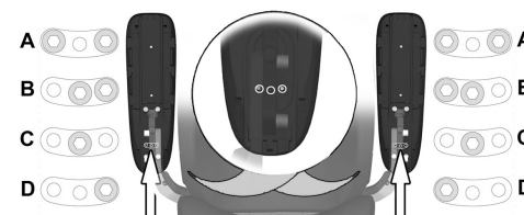
Figure 136. Adjusting the armrest swivel end position.
