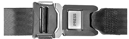
Figure 158. Belt buckle locked properly in the snap lock.
