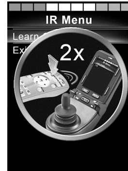
Figure 71. Point the remote control at the IR receiver. Press the button twice.
