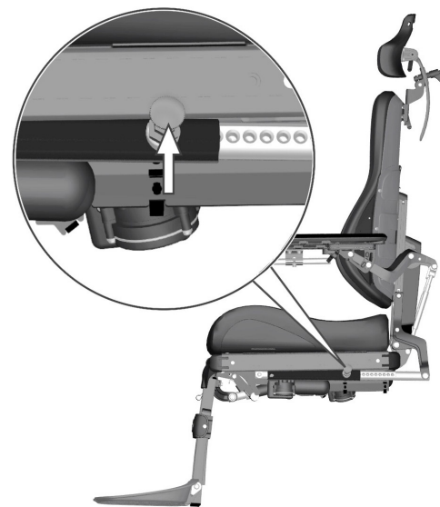
Figure 19. Manually adjusting backrest angle.
