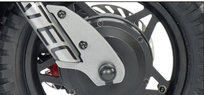
Removable right dropout to change inner tube and/or tyre easily.
