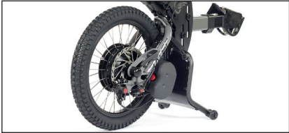
18” Wheel, ultra-grip tyre and aluminium double-wall rim.
