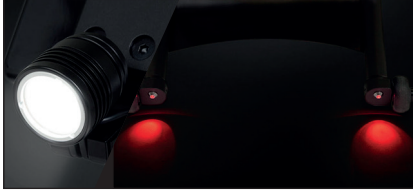
700-lumen front light with position lights / high beam options. Dual LED tail light on the stand frame.
