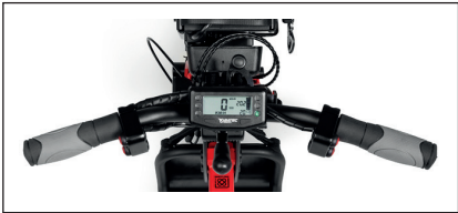
G&B handlebar option without levers for quadriplegics.
