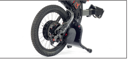
Ultra-grip tyre 18" x 2.40". Black double-wall aluminium rim.
