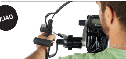
BATEC SHIFT LEVER. Shimano REVO 8 gear shifter.
